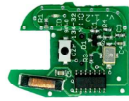
RNR121 ID: 46 RENAULT: Symbol, Clío II, Kango II SCHEDA RADIOCOMANDO 1 TASTO PCF7946 - 433MHZ PROFILO : NE73
