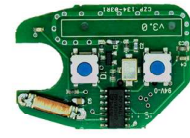
RNR122 ID: 46 RENAULT: Kangoo II, Master II, Traffic II OPEL: Vivaro, Movano SCHEDA RADIOCOMANDO 2 TASTI PCF7946 - 433MHZ PROFILO : NE73
