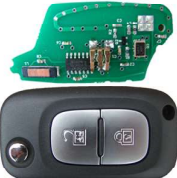
RNR125 ID: 46 RENAULT: Clío III, Kangoo III, Master III OPEL: Vivaro - MERCEDES: Citan CHIAVE RADIOCOMANDO 2 TASTI PCF7947 - 433MHZ PROFILO : VA2
